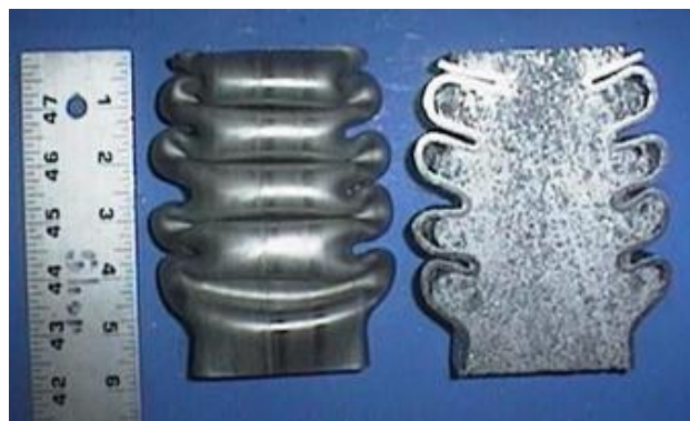
Figure 3. Stainless steel tube with adhesively bonded aluminum foam insert, tested in axial compression to 58% strain
