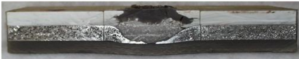
Figure 4. Cross-section through lightweight composite integral armor using layer of aluminum foam
